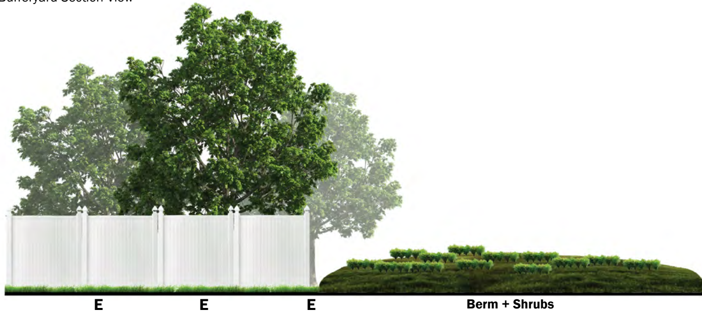
FIGURE 3.9 - Heavy Bufferyard Section View
